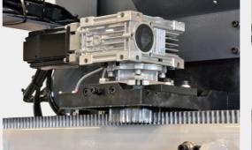
Precision rack and pinion with servo motor driving
